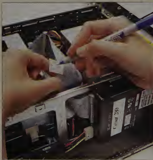
MAKE A NOTE of how all those flat gray ribbon cables connect to various drives.
